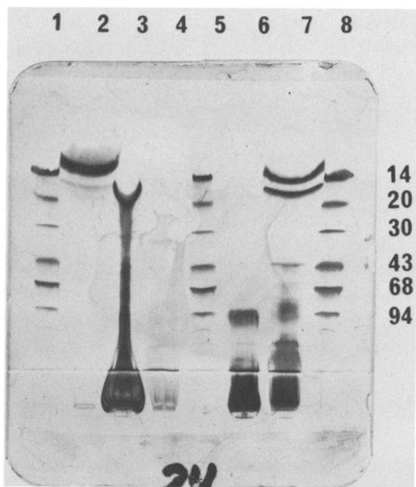
Fig. 2. SDS-PAGE of fractions A–D in Fig. 1 (lower panel). Lanes 1–8 show the separation in 8–25% gradient. SDS-PAGE gels (separation range 8000–200 000 daltons) of molecular weight markers (lanes 1, 5 and 8), fractions A (lane 2), B (lane 3), C (lane 4), D (lane 6) and the total eluate collected from 0 to 60 min (lane 7).
